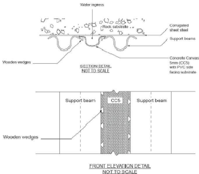
Figure 39. the detailed design of the adopted solution.
